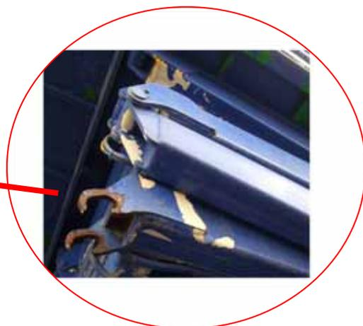
Initial examination identified oxidization, a suggestion of developing fatigue and final stress fractures as shown in *Fig 3*.
