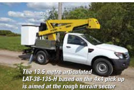
The 13.5 metre articulated LAT-38-135-H based on the 4x4 pick up is aimed at the rough terrain sector
