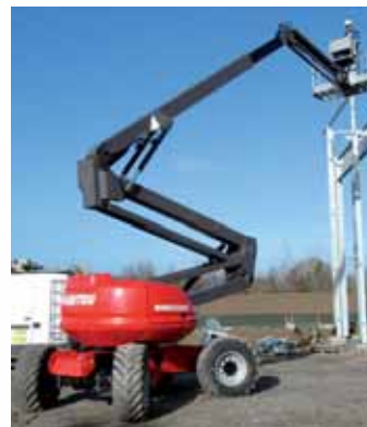
The new 200ATJ shares many components with the smaller 180 and has a 20 metre working height.
