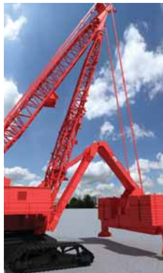
The 31000 includes the Variable Position Counterweight (VPC) which automatically extends when more counterweight moment is needed during the lift.
