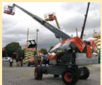
Seen for the first time at a UK show is Skyjack's SJ66T with 20.1 metre platform height and 17.4 metre of outreach.
