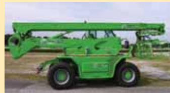
The high-speed Merlo MPR access platform is based on the proven Roto telehandler combining 40 km per hour travel speed with a platform working height of up to 30 metres.
