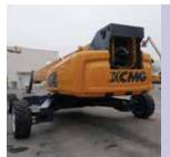
A new 70 metre articulated boom lift from XCMG is spotted at its plant in China. At 224ft it is the world's largest self-propelled boom lift.
