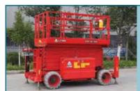
LGMG adds the 46ft SR1418E battery electric Rough Terrain scissor lift with 365kg capacity and 1.52 metre deck extension.
