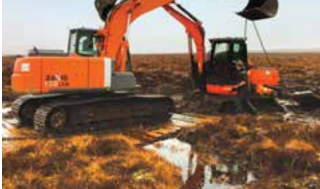
A stricken excavator rescued using timber mats
