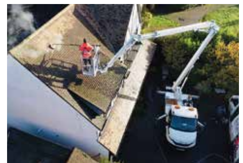
The Aspen A-62 has up to 20.6 metres of vertical reach below deck height
