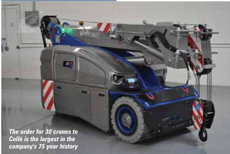
The 20 tonne Valla V210R tops the company's latest generation of battery powered pick & carry cranes
