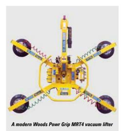
Wheeled stabilisers allow the robots to lift more while remaining compact and help reduce the risk of toppling over sideways on an imperfect surface or from a swinging load. An adjustable glazing head frame also allows it to fit the size of the glazing to be lifted.
