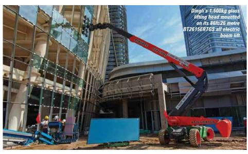
seen the introduction of many interesting and innovative products including Chinese aerial lift manufacturer Dingli's 1,500kg glass lifting head for its 86ft/26 metre BT2615ERTGS all electric boom lift.
