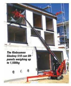
that can be used for placing glass panels up to 1,500kg. The tracked unit can also pick and carry the panels weighing up to 600kg using its side mounted vacuum lifter. Overall weight with 200kg suction head is 2,650kg. Maximum horizontal reach is 7.55 metres with 410kg and it can raise 1,500kg to a height of 7.1 metres.
