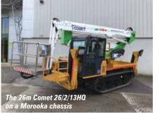
by a two section telescopic boom and articulated jib to offer up to 13 metres of outreach at an up & over height of 11.5 metres.
