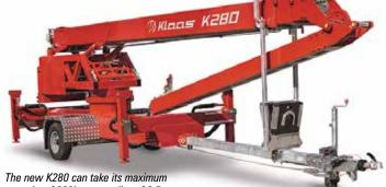
capacity of 800kg to a radius of 6.5 metres
