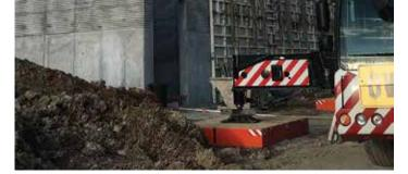
a 50 to 150mm - two to six inch thick layer of sand may be needed. A downside with using sand is that it is messy.
