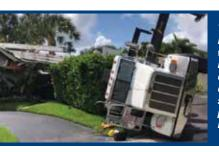
The introduction of outrigger, counterweight and slew position sensing, complete with lockouts, may eventually eliminate this issue while providing improved versatility and ease of setup.
