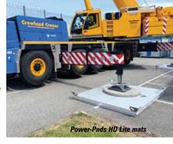
UK based supplier Outrigger Pads is to launch a Inclined Pad range of composite mats that combine with its regular mats to help set up on sloping ground. Its first Incline Pad is 405mm square, with a capacity of 15 tonnes and weighs 12.79kg.
