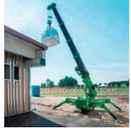
maximum capacity of 800kg. An 818mm manual extension can be added to the jib.
