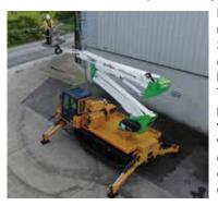
Features include a 250kg unrestricted platform capacity, 360 degree continuous slew, 180 degrees platform rotation and low pressure hydraulic controls. The Morooka MST800VDL diesel powered chassis features 595mm wide rubber tracks, has an overall width of 2.7 metres and four fold down outriggers. Overall weight of the machine is 10.3 tonnes and offers travel speed of up to 12kph.
