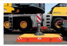
average ground bearing pressure to 5,625psf/26.9 tonnes per square metre which is the objective.
