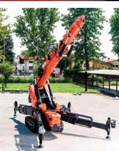
The angle of the beams and the amount of beam extension is completely variable.
