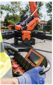
stowed width is 988mm, but the tracks extend hydraulically to 1.38 metres for greater stability on site.
