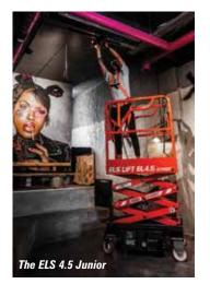
capacity of 120kg, and an overall retracted width of 740mm. But it also has wheeled stabilisers - due to its light weight - which extend the width to 1.65 metres and is all aluminum.
