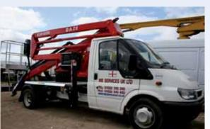
**Allan Access** mounts the first 20 metre lift on a Ford Transit 350, a Socage Appache DA20.
