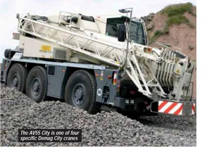
point avoids the typical droop snout of the City crane and provides the crane lifting potential as soon as the boom is raised from the travel position making it ideal for machinery installation.
