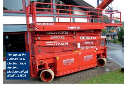
rental company Niken favoured this type of lift mechanism and designed several models which it had made by subcontractors working to its designs.
