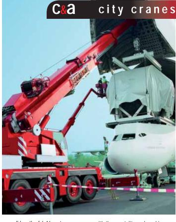
overall length of 6.46 metres, width of 2.19 metres and height of 2.9 metres it is very compact. Maximum travel speed is 40 km per hour and GVW is 18 tonnes.
