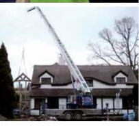
was regularly hiring in mobile cranes from 15 - 50 tonnes, sometimes as big as 200 tonnes primarily to achieve the required boom length. Now, all the high level lifting is done using Böcker trailer lifts. Power Lifting Services has four trailer cranes in its fleet - the 1,200kg capacity, 27 metre lift height AHK 27 and three 31 metre, 1,500kg capacity AHK 31s. The main difference between the two is that the AHK 27 has a two section boom with the larger machines three sections.
