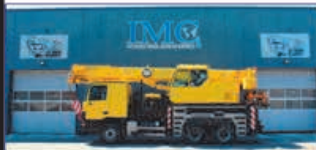
30 t, Liebherr LTF 1030, 2000
