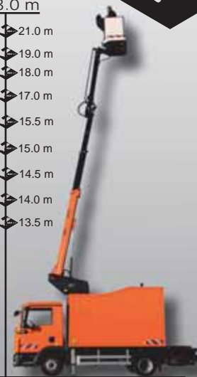
Versalift VT Heavy Duty < 265 kg Korblast > 5.0 T GVW
