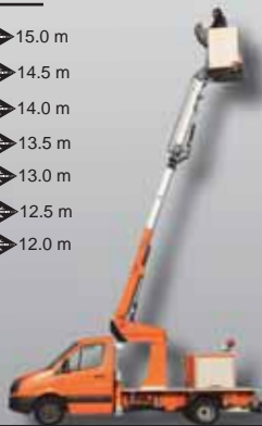
Versalift ETM Medium Duty < 230 kg Korblast 3.5-5.0 T GVW
