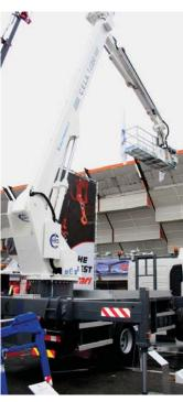
Cela showed its new T350, a 35 metre working height machine with up to 26 metres of outreach. Not many large Cela machines are seen in the UK but about eight fire fighting machines are now with the London Fire Brigade. Currently its biggest model is 54 metres although a 65 metre platform is scheduled for next year's SAIE.
