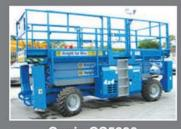
Genie GS5390 diesel scissors 18.5m - 2005/6/7
