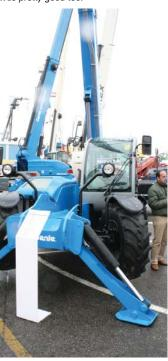
Genie has introduced the the GTH4017SX - a lower cost, simpler machine aimed specifically at the rental market.
