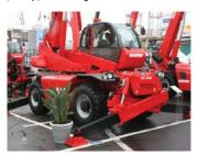
Several new Privilege series from Manitou were on the stand including the roto MRT 2150 (above) which can lift up to five tonnes to 20.6 metres, and the MRT 3050 which can take the same load to 29.7 metres. Largest machine on the stand was the 21 tonne capacity MHT 10210.
