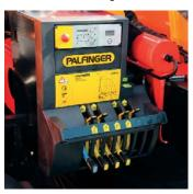
The easier to use Palfinger control panel.
