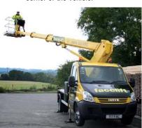
This is as far as the boom will rotate to the offside of the machine.
