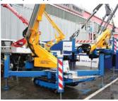
Not currently available in the UK - mainly the Middle East and North Africa - are the co.me.t truck mounted and spider machines. The company produces three crawler models - 12 metre, 16 metre and 18 metre. It was also showing a new 19 metre, 3.5 tonne truck mounted Eurosky AT.
