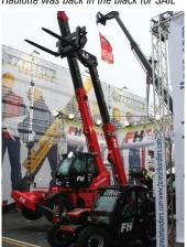
Faresin showed two new models - the 15.45 a 360 degree roto machine and the 6.25 compact model. Improved visibility to the right side of the machine is aided by a redisgned engine cover.
