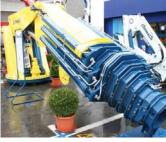
A massive new 200 tonne/metre articulated loader crane from Cormach the 225000 E9 - has been designed specifically for industrial moving. The nine section beast has a 45 tonne lift capacity at 4.5 metres and is capable of lifting 6.1 tonnes at 23 metres and taking more than a tonne out to 42 metres.
