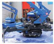
Leader also showed a 16 metre spider lift called the Jumper 160, the first two of which have been sold in Holland. The new model features an unusual crawler chassis with a raised drive sprocket and pinion mounted bottom rollers which allow the lift to travel over obstacles without the mid track tip problem that occurs on many tracked machines.
