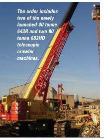
Inverness-based Weldex has bought four Sennebogen telescopic crawler cranes supplied by UK distributor EH Hassell. The order includes two of the recently launched 40 tonne 643R telescopic crawler and two 80 tonne 683HD telescopic crawler machines. Both models are the first to be sold in the UK - the 643R superseding the 40 tonne 630RHD.
