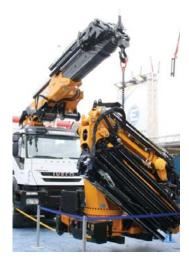
Effer unveiled two new loader cranes: The, 92 tonne/metre Effer 1355/9\$ (mounted) features X-type outriggers which keep the sub-chassis shorter and also gives a better load slewing range. Being lifted is the 470/6S - a six extension unit with a 41.6 tonne/metre capacity and an outreach better than 26 metres.
