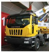
TCM showed its new C2000 - a compact 200 tonne crane mounted on a four axle Astra truck with an overall length of just 10.5 metres.
