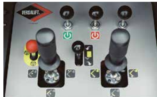
The new fully hydraulic twin joystick control system.
