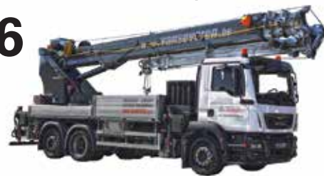
The new Böcker AK46-6000 on a MAN TGM 26-290 three axle carrier.
