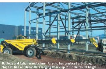
Haulotte and Italian manufacturer Faresin, has produced a 6-strong 'Top Lift' line of telehandlers ranging from 7 up to 17 metres lift height and up to 4 tonnes lift capacity. Pictured is the H17.30.
