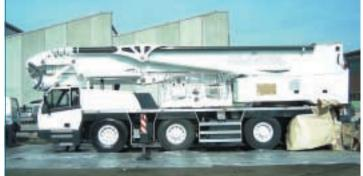
The latest truck mount from Oil & Steel, launched at Intermat, is its 76 metre working height Stargate 7638. The unit is mounted on a 4-axle, all-steer chassis and provides a 38 metre working radius.
