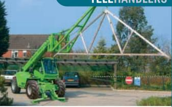
Merlo has introduced attachments specifically designed to permit its telehandlers to travel with the boom lowered while transporting roof trusses on site.
