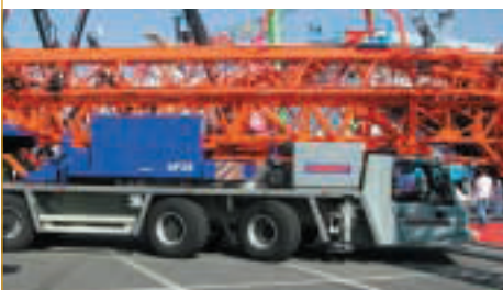
Pictured is Arcomet's new 6 tonne capacity AF 38 truck mounted self erecting tower crane mounted on a Tadano Faun carrier. The unit carries a 38 metre maximum boom length where it can lift 1.8 tonnes.
