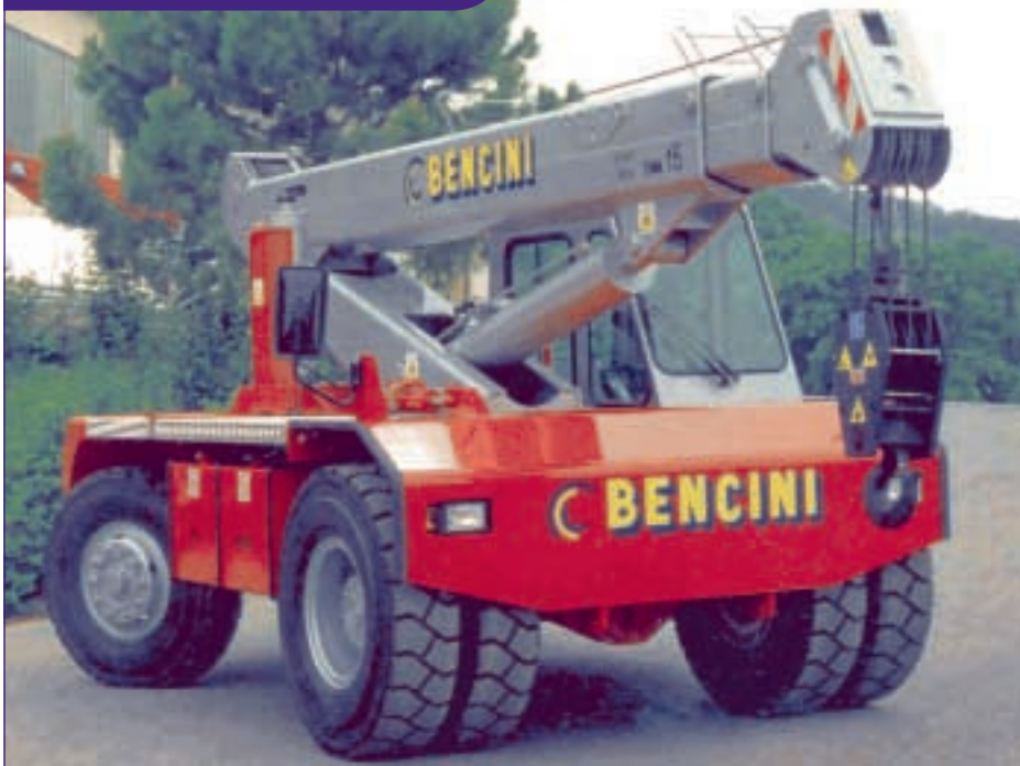
Above: Italian producer, Cams Industriale, manufactures self-propelled industrial cranes under the Bencini logo. Pictured is the 15 tonne capacity, overhauled version of its SP150 model.
