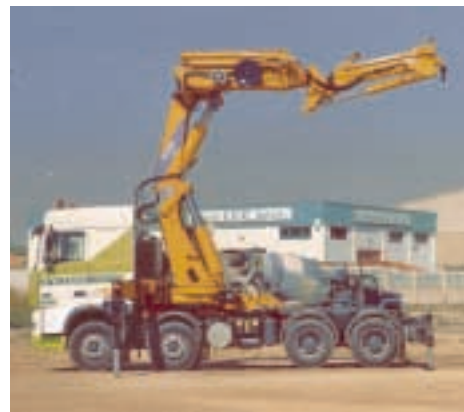
All new large Effer knuckle boom feature continuous slewing, which Effer says is how it defines its large knuckle boom cranes. Pictured here is its 135 tonne/metre 1350 model.
