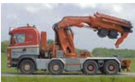
This 150 tonne/metre F1500AXP from Fassi is available in three basic versions and is now company's largest knuckle boom unit.
