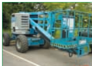
SELF PROPELLED TELESCOPIC PLATFORM 1998 GENIE Z45/22 15m. working height (50ft.). Deutz Diesel Choice of 20 machines.
