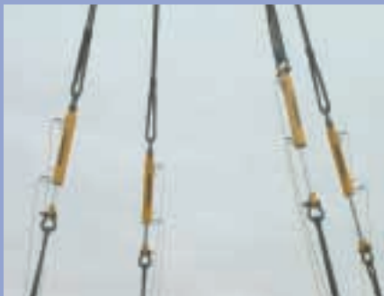
Accurate load positioning is done using four SyncHoist cylinders attached between the cables and the load.
