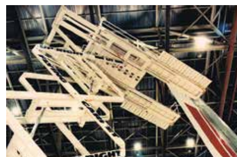
A 47ft Upright Flying Carpet designed for Boeing to work on the new 767, 757 and 747 aircraft including castered hydraulic outriggers, aircraft bumper package and 17ft hydraulic extension platform designed to fit the contour of the vertical stabiliser
