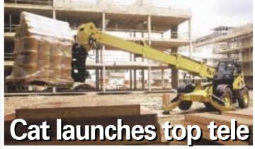
Caterpillar has topped its telehandler line-up with the introduction of what is now the company's largest model. Allocated the TH580B, the new unit is rated at 5 tonnes capacity with a maximum lift height of 17 metres, and completes Caterpillar's eight-strong B-Series telehandler range up to 5 tonnes lift capacity and lift heights up to 17 metres.
