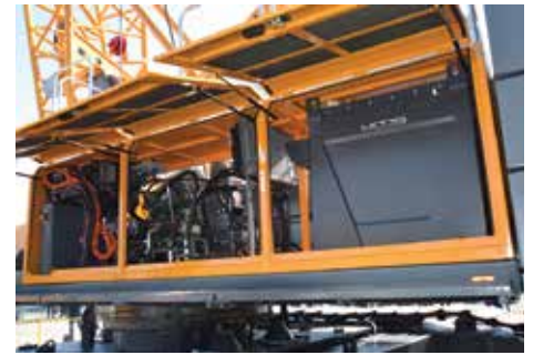
Marchetti's new hybrid power system for its Sherpina cranes offers Battery, diesel or plug-in power
