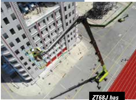
ZT68J has a 67.7m working height
