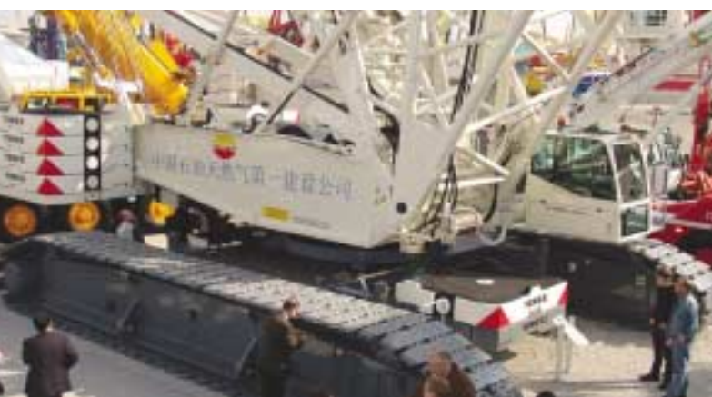
Terex-Demag targeted the wind energy sector with the launch of its 350 tonne capacity CC 2200 at bauma 2004.
