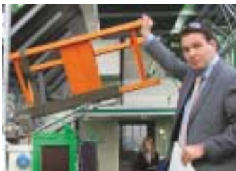
Stefan Salvia of Rovers demonstrates how with one hand and wearing a suit, he could install mast sections.
