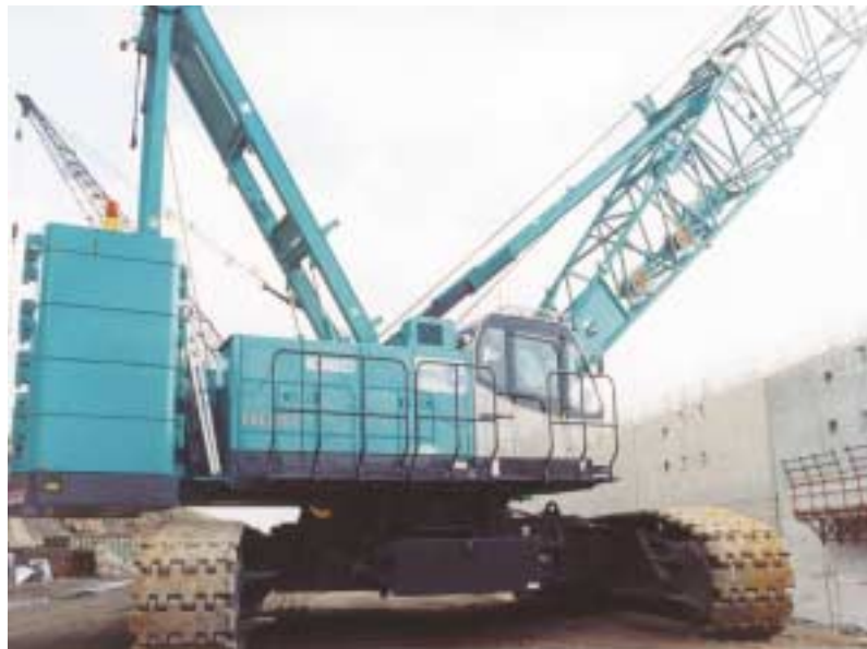
One of Kobelco's latest crawler releases first seen at bauma earlier in the year – this 135-tonne capacity CKE1350 has been put to work by owner Benelmay on one of Europe's largest construction sites, the Deurganckdok container terminal in Antwerp.
