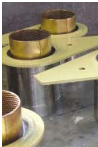
Holland Lift takes no chances and supplies Scissor Arm Pivot Pins with dual lubrication tracks (right). The pins also sit inside substantial bushes which in turn sit inside heavy duty collars (left).
