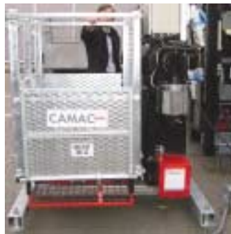
Camac's 90-degree pinion drive arrangement makes this lift compact enough for a 1.5- x 1.5- metre lift shaft.
