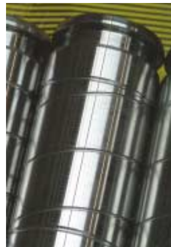
Holland Lift takes no chances and supplies Scissor Arm Pivot Pins with dual lubrication tracks (right). The pins also sit inside substantial bushes which in turn sit inside heavy duty collars (left).
