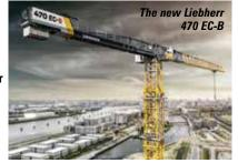
capacity on the 16 tonne version is 3.2 tonnes reduced to three tonnes on the 20 tonner. A three metre jib extension takes the maximum radius to 83 metres, at which point jib tip capacities are 2.4 and 2.2 tonnes respectively.
