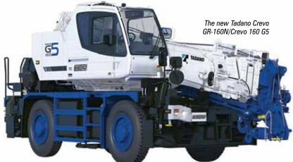
the crane for improved visibility when travelling - particularly in urban areas when driving alongside cyclists and pedestrians - and incorporates a 'Human alert system' that detects and warns the driver when people are near the crane, both on the road and on site.
