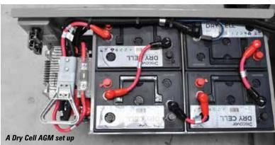
such as aerial work platforms. Like the AGM battery the charger needs a specific Gel setting to avoid overcharge damage. And the charger and charge algorithm should support temperature- compensated charging.
