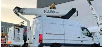
One of Klubbs latest releases is the 19m KT18PZ mounted on a seven tonne van chassis which claims the best working height of any van mount
