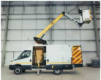
in the region of 17 metres. Although the larger vans need additional driving licence requirements for younger operators, their main advantage is the much larger cargo carrying capacity - up to 2,300kg when mounted on the largest chassis.
