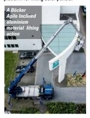
Both of Klaas's models - the Toplight 21 Construction and HV 26/6 KA are trailer-based, as are Böcker's Simply, Junior, Avario and Junior G units. These can lift a little more and a little higher: the Avario, for example, lifts 270kg and reaches 27 metres. Material lifts like these are a common sight in many cities in mainland Europe.
