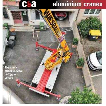
The aluminium was required in order to make lightweight and high performing booms, which gave the possibility of a high reach. But today, there are steel alloys that have the same, and even better, characteristics in terms of weight lifting and reach performance. So that is why with certain models, we have made a transition to steel booms."
