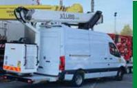
launches its highest working height van mounted platform to date - the 19 metre KT18PZ
