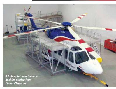
Because of the design of the bay, outreach is also needed. Access manufacturers often work with the major aircraft manufacturer to supply specially modified equipment such as mast booms to gain access to this area of the aircraft. Push around platforms are also used in both the front nose wheel bay and main undercarriage bay areas.
