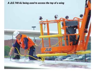
repair when the full cost of repairs, retesting and most importantly downtime are taken into account. Simple padding and buffers helped but were not an ideal solution. Over the years however, aerial lift manufacturers have developed and improved their hydraulic systems and controls and today supersmooth proportional control drive and lift functions are prerequisite, making them ideal for the fine
