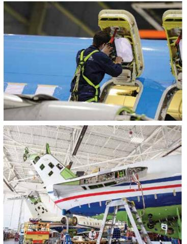
hangar door for the tail access. The tapered design reduces construction costs and heating what would be empty space. This system works especially well if the hangar is dedicated to one aircraft type. In a number of cases the tail docking is suspended from the roof and can slide in and out to allow the aircraft to exit the hangar. Access via staging to the fuselage and wings can either be of a fixed or mobile design.
