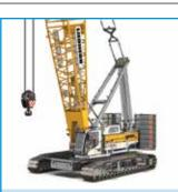
Liebherr launches its first battery electric lattice boom crawler cranes - the 200 tonne LR 1200.1 Unplugged and 250 tonne LR 1250.1 Unplugged.
