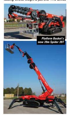
and it can be ordered as a diesel/lithium-ion hybrid or with diesel/AC electric power. It joins the company's 30 metre Spider 30 T and its 43 metre 43 T.
