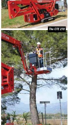
power is Kubota diesel, which is available with an additional AGM battery pack, good for around an hour's continuous operation. It can also be operated while plugged in and recharging, so in essence three power sources on the same machine.
