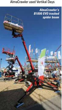
to launch its new UK subsidiary -Almac Atlantic - as well as unveiling the new 18 metre B1890 'Spider Boom', the first in its Billennium Quick-Pro range. The telescopic boom and articulating jib provide a maximum outreach of 10.9 metres with 80kg in the basket, while 8.1 metres is possible with the maximum 250kg. Power comes from a Yanmar diesel.
