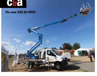
Sinoboom's UK dealer Pinnacle Platforms launched the 46ft AB14E and 53ft AB16E all electric articulated boom lifts. Apparently new battery powered RT scissors and mast type lifts are on the way. GSR unveiled its new 20 metre B210PXJ articulated truck mount with 2.4 metre jib and 250kg platform capacity, one of 10 sold to Smart Platform Rentals on a 3.5 tonne Mercedes Sprinter chassis. The show was the first chance to
