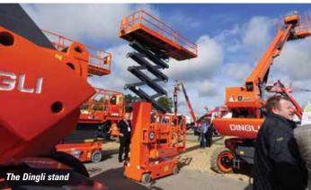
a new 46ft AR14J for Quick Reach. The Dingli stand was a sea of orange, exhibits included the battery powered 4x4 66ft BA22ERT articulated boom lift, with a 22.2 metre working height and 12.7 metre outreach with 230kg platform capacity.
