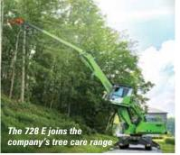
its maximum capacity at 4.5 metres and 1.7 tonnes at a radius of 18 metres, while offering up to 7.5 metres below ground reach. Features include a 2.7 metre elevating cab and a wide range of attachments.
