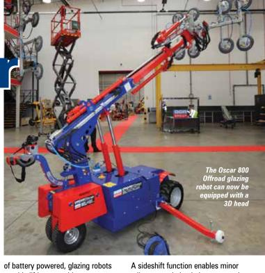
provide lifting capacities up to 1,400kg.
