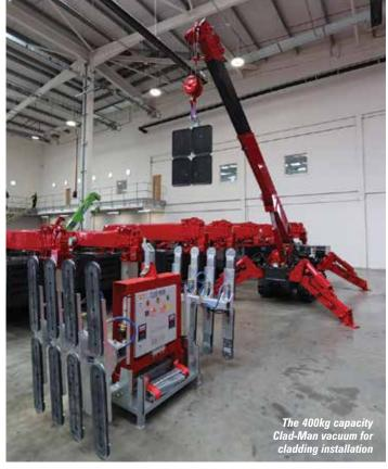
It is operated by a Hetronic radio remote control system, and it can lift canopy glazing to a maximum height of 4.25 metres in the vertical plane, or 2.7 metres when glazing horizontally overhead.
