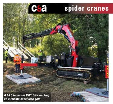
calling the TMC525, as part of its UK branding. It has a maximum tip height of 20 metres on the eight section main boom, while a six section iib takes this to 32.5 metres and out to a radius of 29.4 metres. In fact, it offers 12.6 metres of horizontal outreach from the main boom nose at an up & over height of 20 metres.
