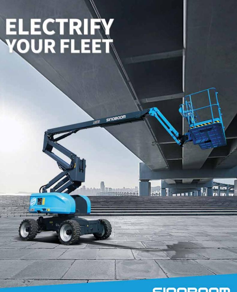
With zero emissions and quiet operation, Sinoboom electric-powered articulating boom lifts deliver long-lasting performance both indoors and outdoors. Our intelligent display screens provide easy viewing of machine status and trouble shooting. Max working height from 16m (52'6") to 20.2m (66'3").
