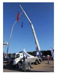
weight manoeuvrable long reach cranes are proving ideal for handling roof trusses, small cooling units, and a wide range of similar work. "The advantages of these cranes really stand out on the road," says Marnock. "They're so cheap to run, compared to 50 or 60 tonne All Terrains."
