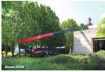
lithium-ion battery pack, but that it has an all electric tracked chassis with IP67 permanent magnet direct electric drive motors. Hinowa claims that the concept is four times more efficient than the traditional hydraulic motor driven tracks, while also significantly reducing the amount of hydraulic oil on the machine, particularly in the chassis.
