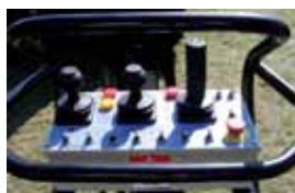
The Haulotte controls were one of the few that use joysticks for all functions.
