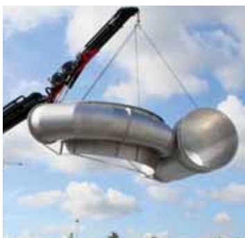
The 72 tonne/metre Thor is the largest machine produced by HMF, here seen lifting parts for a food processing plant in the port of Aarhus. The machine is fitted with the EVS stability system.
