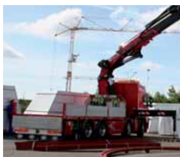
The 72 tonne/metre Thor is the largest machine produced by HMF, here seen lifting parts for a food processing plant in the port of Aarhus. The machine is fitted with the EVS stability system.
