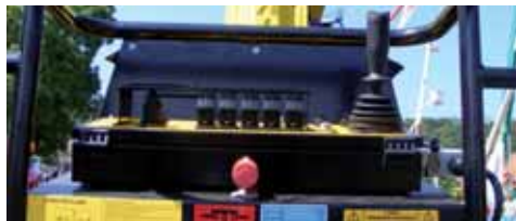
The Airo controls were well protected and had a vinyl cover to provide extra protection in wet weather
