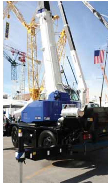
Not available in Europe, the compact Tadano GR150XL is more of a city crane than true RT.
