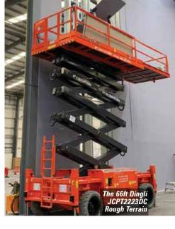
Last spring, leading Chinese manufacturer Dingli launched two 66ft heavy duty battery powered scissor lifts. The 2.3 metre wide JCPT2223DC is an electric version of the classic diesel RT model but with a tight narrow scissor stack. This allowed it to be used on the 1.25 metre wide slab electric JCPT2212DC narrow aisle version. As a result, Dingli is possibly the first manufacturer outside of the Netherlands or Germany to enter this ultra-niche corner of the scissor lift market.
