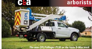
on a 3.5 tonne chassis. This unit offers up to 8.2 metres outreach. with a platform capacity 200kg which may be a little light for some arborist's work. However, from the Klubb line, CPL can fit units in the KT range on the 3.5 tonne lveco Daily, with working heights from 17 to 20.6 metres, up to 12.5 metres outreach and 300kg platform capacity.
