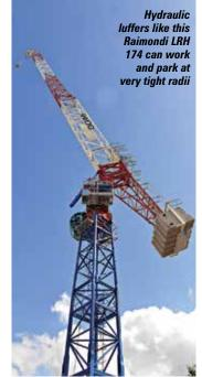
Traditional luffers competed with saddle jib tower cranes and climbing derricks on skyscraper construction, not for maximum radius, but for their ability to reach high, without needing a very high tower or frequent climbing.
