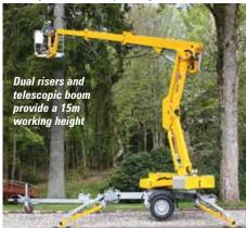
On the road, the overall width is 1.66 metres, with a length of just over six metres, while the stowed height is just under two metres. The AC mains or lithium-ion battery powered models have an overall weight of 2.000kg, including hydraulic outriggers and hydraulic drive assist for manoeuvring on site. The standard lead acid battery pack adds 50kg. Options include radio remote controls, diesel or petrol power.
