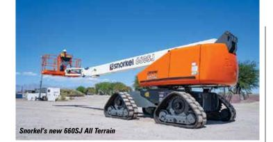
dubbed the 600/660SJ All Terrain. They offer a maximum outreach of 16 and 17.8 metres respectively with 272kg/454kg platform capacity. At the same time Genie has updated its TraX product range with the already mentioned S-80 J TraX, and European version of its 62ft Z-62/40 articulating boom, taking its TraX range to six models.
