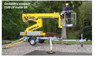
up and over height of almost five metres. The lift has 400 degrees of slew, while platform rotation is 100 degrees. Overall operating width with the outriggers set is 4.12 metres.
