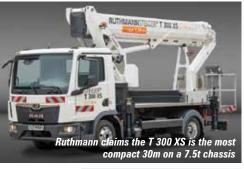
in the T series, the T 300 XS will feature the company's new outrigger set up controls with automatic monitoring and envelope calculation. It can be supplied with a range pruning, insulated and extra wide platforms.
