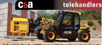
Fork pockets allow the 1.250E power pack to be easily moved around on site
