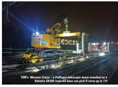
attachments, there are times when more capacity or reach is required. Each of the suppliers I spoke with cater for this need, including SRS's Palfinger on its purpose built carrier, with extendable counterweight.
