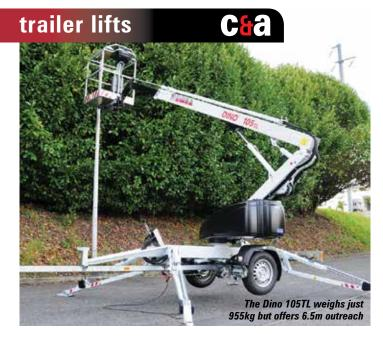
with 130kg platform capacity. The low weight amazingly includes hydraulic outriggers and a wheel drive assist system! The 12 metre 12T is also a one person machine, with an unrestricted platform capacity of 120kg, but offers 7.9 metres of outreach, weighs 1,285kg fully equipped, and has an overall length of 5.56 metres.
