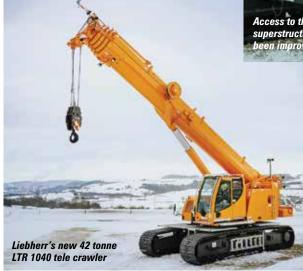
The LTR 1040 has an overall weight of 43.5 tonnes, including its 5.6 tonne counterweight and hook blocks. Its retracted tracks extend from three metres to 4.8 metres with intermediate working widths. The overall height is 3.15 metres. Buyers will also be able to upgrade the LTR 1040 into an LTR 1060 retrospectively if required.
