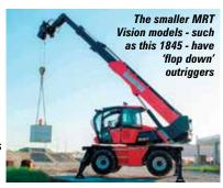
the deck is available on both sides and both ends of the chassis making it easy to climb down regardless of the superstructure slew position.
