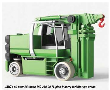
Tilting the mast forward extends the horizontal reach to five metres, with a capacity of 5.6 tonnes, although the lift height is reduced to just over seven metres. The maximum 25 tonnes capacity is available 500mm in front of the machine and, as with all capacities, is available at full height.
