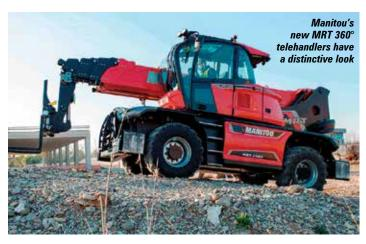
The new models feature all new high vision cabs with no structural cross bars to restrict the view. The cabs also feature an extra large touch screen with pop up informatics and a hot water heater. The new machines are said to be up to five percent lighter than existing MRT models yet offer capacity improvements of up to 15 percent. Access to
