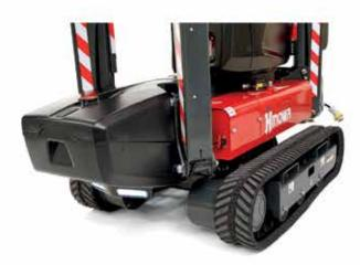
OUTRIGGER PADS HOLDER AND LED FRONT AND REAR WORKING LIGHTS
