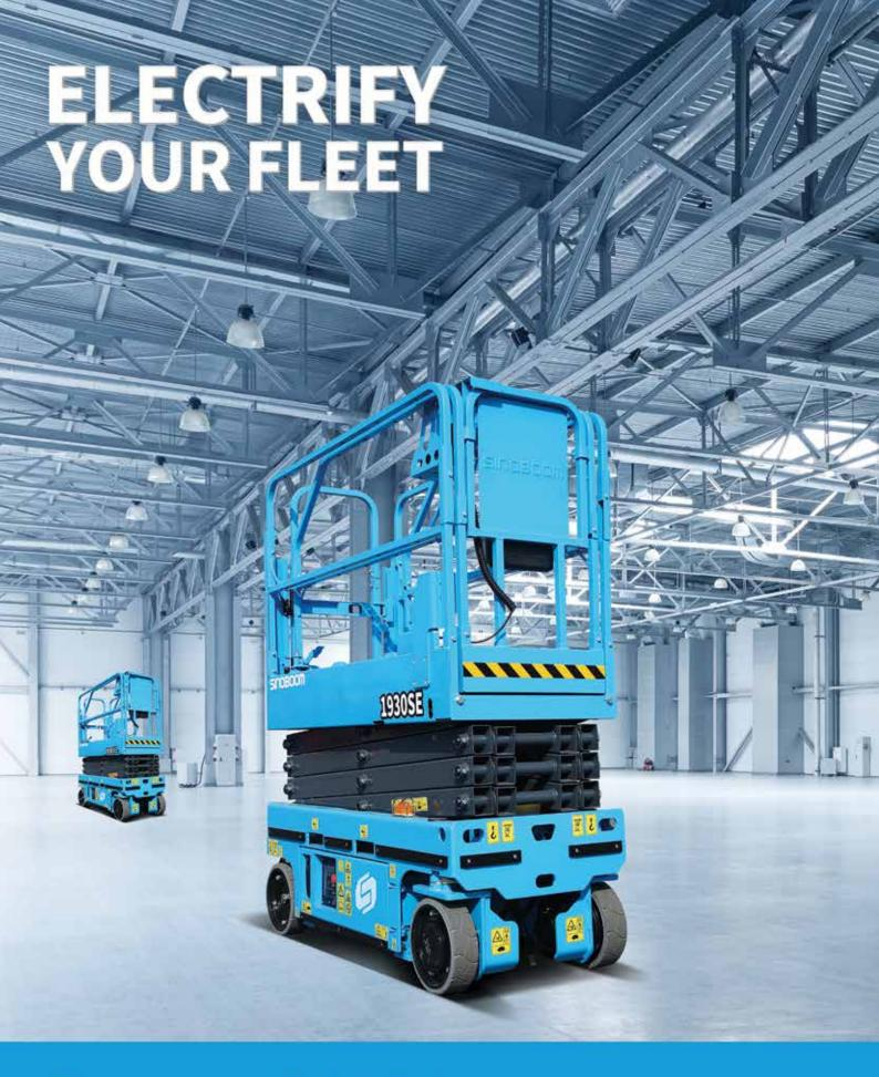
Efficient and environmentally friendly, the Sinoboom electric scissor lift series features platform heights from 4m (12'6") to 14m (45' 3") and offers numerous benefits: exclusive open chassis design for reduced daily maintenance time; bumper rail protection; lower cost of ownership and highly versatile parts and components.
