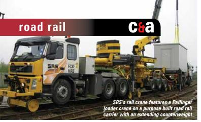
post or tree handling or signalling. Each has its own specialised lifting requirements. Excavator and telehandler based machines can use different attachments to match the work. SRS, however, takes a different approach with a modular system, using a standard container locking mechanism to attach the equipment. This allows various machines to be quickly swapped as required, for example switching between a loader crane to the flat cargo deck of an aerial work platform in minutes.
