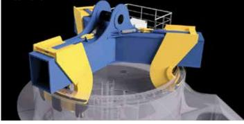
nine cameras, giving feedback to the crane cab, helping operators work safely, swiftly, and efficiently. The remote controlled attachment is equipped with a small diesel engine,
