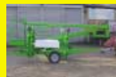
NIFTYLIFT I20HE (1998) Trailer mounted platform. Hydraulic jacks. 40' working height. Battery. Repainted, serviced & tested.
