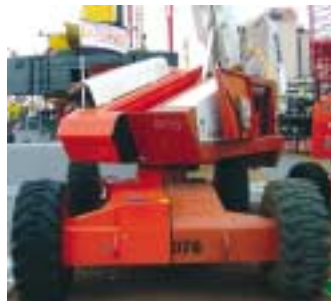
"Snorkel used a Unique half and half way to show how it refurbishes old boom lifts at its St Joseph plant"
