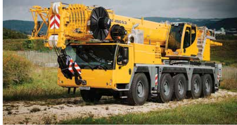
Liebherr's new LTM 1150-5.3's features a 66m boom, the longest on a 150t crane
