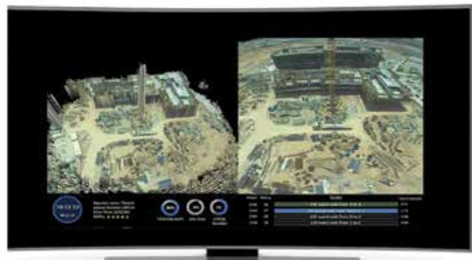
The system can be used to provide visibility and monitoring functions of the site in both 2D and 3D
