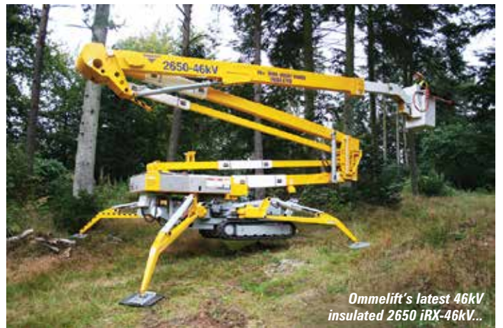
..with a hydraulic circuit for saw hook up
