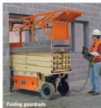
floor loadings are often important for these small machines. One of the big selling points of Hy-brid Lifts over the years has been the ability for its machines to work on suspended floors thanks to their ultra-low overall weight.
