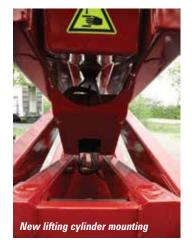
are highest. The changes have significantly lowered the machine's centre of gravity while reducing the weight of the scissor stack, so that it is now a good deal easier to extend. This has also lowered stress levels throughout the upper areas of the lift mechanism.
