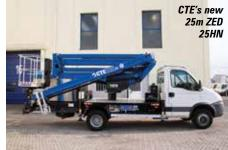
'H' type Narrow outrigger set up - has only jacks, with no outrigger extension beams. The Zed 25 HN offers a maximum outreach of just over 12 metres at an up & over height of 10 metres with a reduced 100kg platform capacity while maximum platform capacity is 250kg. The first unit has been delivered to the cleaning and maintenance division of Slovakian manufacturer TreeGuard.
