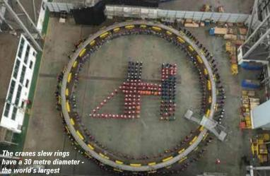
which can handle 70 tonnes at a mere 12 metres radius, or 25 tonnes at 60 metres!
