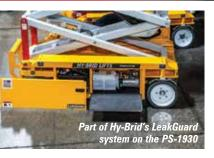
have electric drive, electric steer and sealed batteries and the only fluid on board is that used for the lift cylinder with the Hy-Brid machine having a built in drip tank and small absorbent mats all of which it promotes under the 'LeakGuard' name. The Snorkel also incorporates most of the lift cylinder hydraulics into the lift cylinder module, an idea pioneered by JLG with its initial ES series almost 20 years ago.
