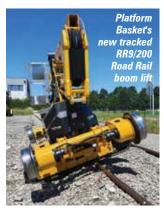
The superstructure also includes automatic levelling allowing it to level up
