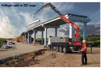
Tec 7s - DPS Dual Power System for full lifting power in jib mode - DPS-Plus for the TEC 5, and DPS-C for the TEC 7 - along with the HPSC-Plus module which monitors the crane bed tilt to provide increased capacities and improved stability by taking the load on the truck into consideration. This allows higher capacities when fully laden which reduces as it is unloaded.
