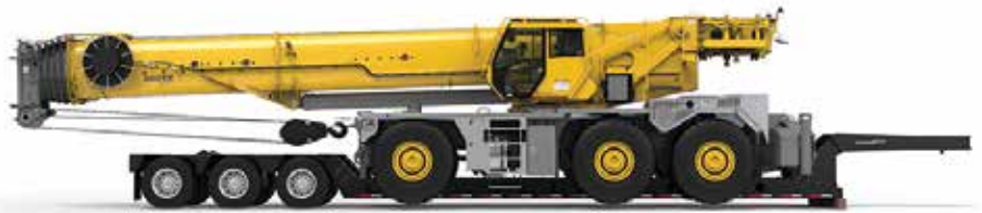
The new GRT 9165 is said to be easy to transport on a beam trailer having an overall travel height of 4.23m.
