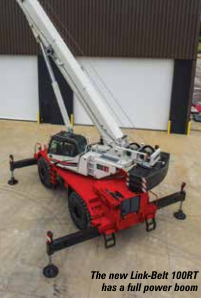
The Link-Belt 100RT incorporates V-CALC (Variable Confined Area Lifting Capacities) which features 12 different outrigger configurations with real time 360 degree charts.
