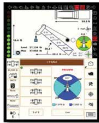
The Link-Belt 100RT incorporates V-CALC (Variable Confined Area Lifting Capacities) which features 12 different outrigger configurations with real time 360 degree charts.
