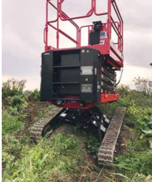
The crawler scissor such as this Almac Bibi BL-1090 is a possible alternative for an RT scissor
