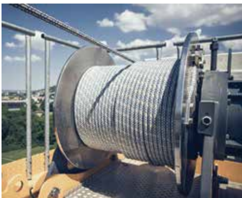
The new fibre rope from Liebherr.
