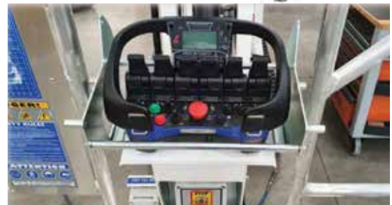
The new Scanreco remote controller in the basket cradle.
