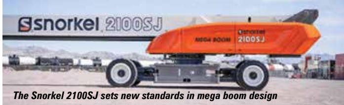
The 2100SJ'S unique chassis with 'drive out' extension arms.
