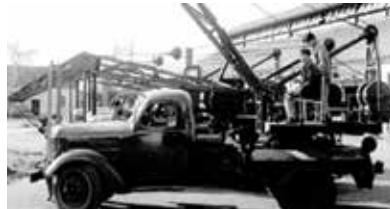
XCMG's first wheeled crane in 1963 - a 5 tonne truck crane.
