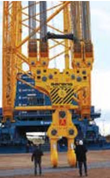
The cranes 3,200 tonne hook block.
