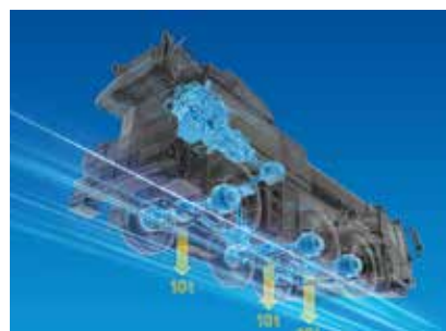
At the heart of the ATF60G-3 is a single superstructure mounted six cylinder Mercedes Euromot IV/EPA Tier 4f diesel.
