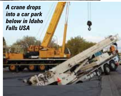
For the Spreader Pad Calculator to work effectively, you will need to know the maximum load per outrigger and the maximum allowable ground pressure
