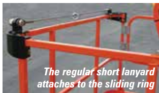
The system allows the operator to work outside of the platform
