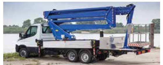
Maximum outreach of the Comet is 17 metres with 250kg platform capacity covering a 240 degree area over the rear and front outriggers
