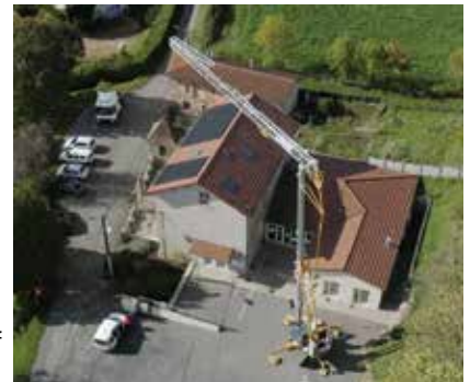
The company claims it is the only self-erecting crane with a 28 metre jib that has such a compact transport format.
