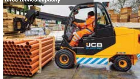
JCB's new C30-19e Teletruck has a four metre lift height with up to three tonnes capacity
