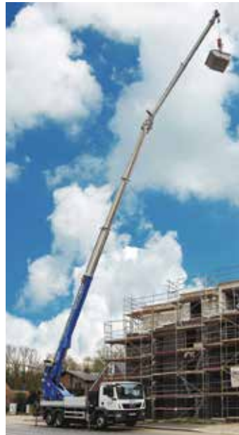
The new Bocker PK 350-D can accommodate up to three people or 350kg
