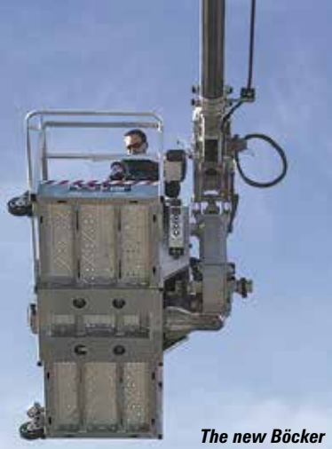
The new Bocker PK 350-D can accommodate up to three people or 350kg
