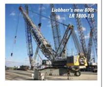
luffing jib can also be extended to 102 metres. Liebherr claims the new LR 1800-1.0 is the most powerful crawler crane on the market with a three metre wide transport width.
