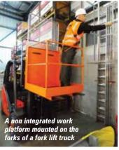
integrated work platforms - ones without controls in the platform - that fit onto the forks where the fork lift driver operates the machine. But note that they are only intended for occasional use when it provides a safer means of access than say improvised stairs, platforms or a ladder or where it is impracticable to use a fully integrated working platform.
