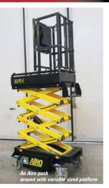
be reduced to a 520mm by 520mm 'micro cage' to work in confined spaces such as through suspended ceiling openings.
