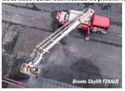
as an aerial lift, fire truck and a rescue ladder. It provides 20 metres of outreach and a platform capacity of 350kg, while the platform has an overall width of 1.8 metres and an overall length of 900mm.
