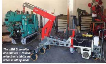
into two push around parts - boom and counterweight/engine - each measuring about a metre long, making the crane very compact, portable and manoeuvrable. With an overall width of just 620mm, it has fold out 1,740mm wide front stabilisers when in lifting mode. Overall length is 2.34 metres with
