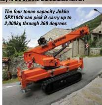
Jekko also has a range of small pedestrian pick & carry cranes and has added lithium power to its two tonne MPK20 and the five tonne MPK50 remote controlled crane/ glass handler. The units currently use lead acid battery packs but can
