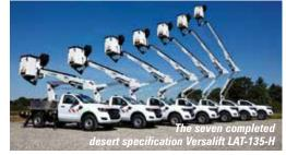
specification 4x4 pickup mounted Versalift platforms.
