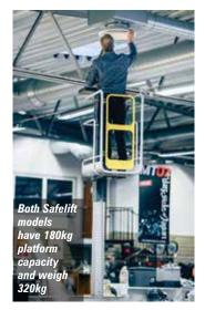
platform measuring 530mm by 760mm, a 16 second lift time to full height and 180kg platform capacity. Overall width is 760mm with an overall length of 1.2 metres and an overall height of 1.64 metres. Both units weigh 320kg.
