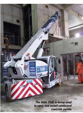
telescopic boom, and a maximum radius of nearly 10 metres. It is also fitted with non marking tyres, the latest 'InTouch' tracking system and advanced remote access diagnostics."
