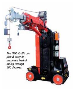
the load has been lifted, the crane can be pushed into position on its wheels.
