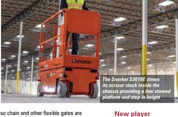
being replaced with European style swing gates. The 1.1 metre guardrail height on CE machines is also a requirement, requiring most 19 and 20ft scissor lifts be equipped with folding guardrails to enable them to travel through a standard door height opening.
