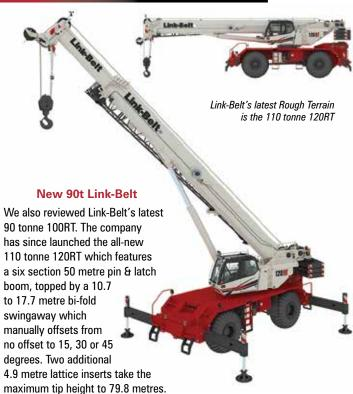
The crane features a Cummins Stage V/Tier IV diesel - or a Tier III Cummins for emerging markets powering a six speed transmission with two axle four link suspension. New ladders and steps give improved access to the carrier deck which now uses slip resistant paint, Link-Belt's V-CALC - Variable Confined Area Lifting Capacities - system features 81 different outrigger configurations and once set, the crane's Pulse 2.0 system indicates the available capacity for the specific configuration.
