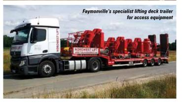
are the same as for 44 tonne C&U (Construction and Use) rules, the requirement to frequently or constantly accommodate 30 tonne payloads requires a heavier trailer construction. The core trailer fleet of many UK access companies comprises trailers from King. Andover and Nooteboom.
