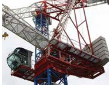
Raimondi's new 18 tonne LR330 luffing jib crane with triangular jib design
