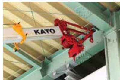
The three tonne searcher hook on the Kato CR-130Rf
