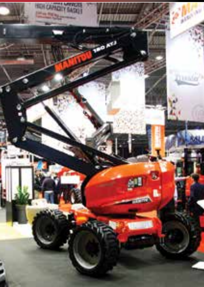
Manitou's third generation 52ft 180 ATJ uses a smaller Kubota diesel engine with LSU pump to extract more performance.
