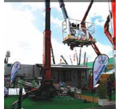
The Hinova Lightlift 33.17 Performance IIS with 16.5m outreach at a height of 17m and unrestricted platform capacity of 230kg and 180 degree jib articulation
