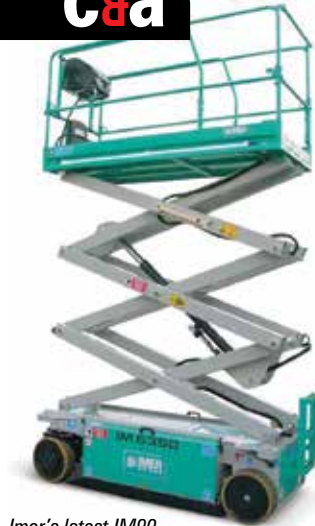
Imer's latest IM90 series includes the 21ft IM-6390.
