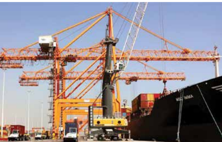
Liebherr ship to shore and rubber tyre gantry cranes.
