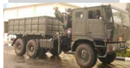
A 6x6 Tata truck complete with material handling crane for the Indian Army.
