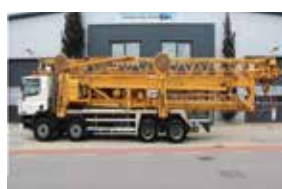
LIEBHERR - MK45 Tower Cranes 6t, 27m Flight 32m Lift Height. DAF Unit 2001 | PHM-Id 09002
