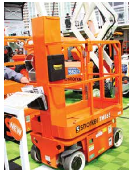
The Snorkel TM16E is a larger 6.7 metre version of the new TM12E
