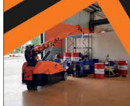
The new Bailey Cranes BC-18 battery powered carry deck crane
