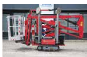
HINOWA - GOLDLIFT 14.70 Track articulating boom lifts Diesel, Tracks, 14.0m Working Height, 2008 | PHM-Id 08704
