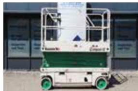
HAULOTTE - COMPACT 12 Scissor lifts Electric, 4x2x2 Drive, 12.0m Working Height, 2006 | PHM-Id 08897
