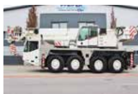
DEMAG - AC80/2 Telescopic Cranes 80t, 8x6x6, Intarder 17.6m Dbl Jib, 50m Boom 2006 | PHM-Id 08852
