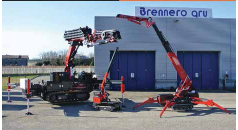
CWE 525: Max hydraulic outreach: m 30 Load capacity Kg 14500 - Easy access: Max width mm 1850
