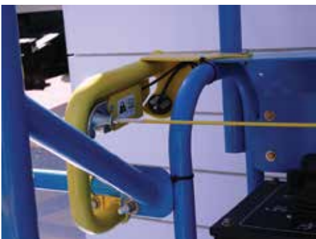
Genie's new 'Lift Guard' Contact Alarm system features an activation cable connected to one side of the control panel with heavy duty magnet.
