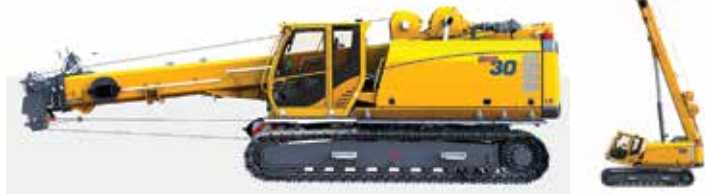
The Grove GCH30 features a three section full power boom.
