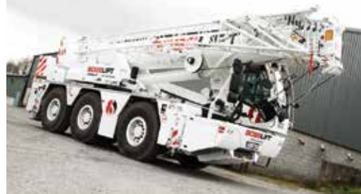
Bosslift's new 50 tonne Liebherr LTC1050
