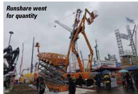
A special airline adapted Huabei scissor lift with lateral slide out deck extension
