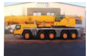
LIEBHERR - LTM1220-5.2 Telescopic Cranes
