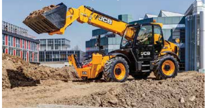
540-140 Hi-Viz - its fourth model in the range which offers better visibility with a lower boom pivot design
