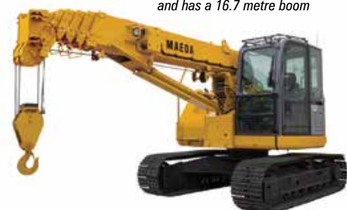
The Maeda CC1485S-1 replaces the and has a 16.7 metre boom
