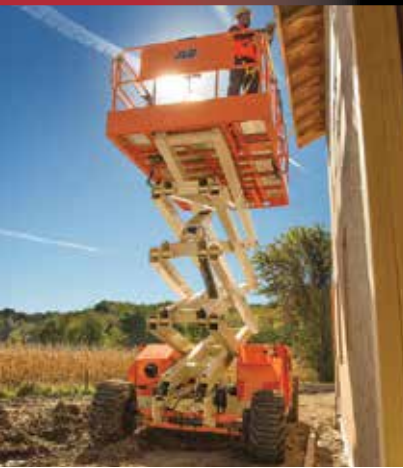
The latest RT scissor lift from JLG is the 53ft 530LRT, with a working height of over 18 metres and 680kg platform capacity.
