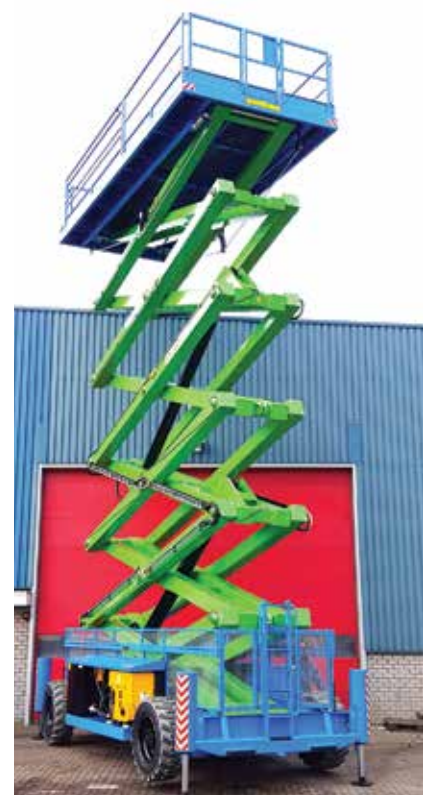
Largest Holland Lift scissor is the three metre wide Megastar HL340-D30 with a working height of almost 34 metres.
