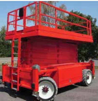
PB Liftechnik has launched a new 67ft heavy-duty, battery electric RT scissor lift. The 22.3 metre working height S225-24ES 4x4.
