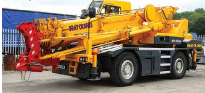
The Kato CR-350RI can pick & carry up to 9.5 tonnes at up to three metres radius
