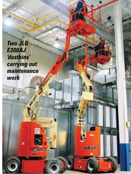
Mastbooms are narrow enough to work between compact aisles
