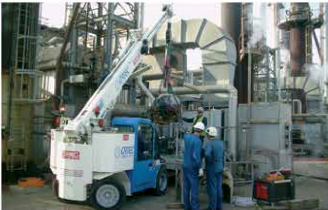
The five tonne MPK50 has a maximum lift height of eight metres
