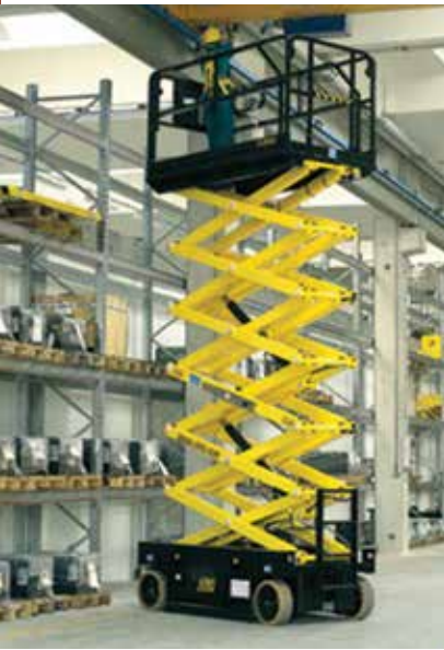
There is another type of platform that will do this task - the scissor lift with a 1.5 metre platform extension such as this Airo 14EW.
