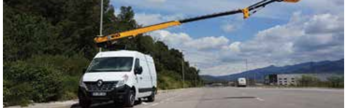
The new 14m Movex is designed for 3.5 tonne vans
